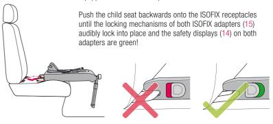
Now reinsert the seat, depending on the age of the child either in the driving direction or opposite to it (see "MOUNTING THE SEAT OPPOSITE TO THE DRIVING DIRECTION (FROM BIRTH TO 13 KG)" or "MOUNTING THE SEAT IN THE DRIVING DIRECTION (FROM 9 - 18 KG)").
