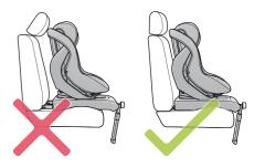
Press the support leg button (09) and move the support leg (10) downwards until it rests securely on the floor and you can hear and feel it lock into position!
