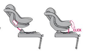
Then fold the seat forward until the front seat lock (11) audibly locks into the ISOFIX base and the safety display (07) on the top is green.
