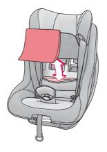
If the child's bodyweight exceeds 8 kg, the pre-mounted pelvic insert should be removed. This can be found in a pocket under the seat, on the reverse of the seat cover.
